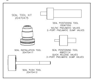
Figure 9-23: Pneumatic Valve Seal Tools
