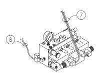
The 4-way directional control valve shifts the hydraulics back and forth to the intensifier. A shift valve directs pressurized oil to one end of the hydraulic cylinder and returns fluid to the reservoir from the opposite end, causing the intensifier to stroke. The movement is controlled hydraulically by a pilot valve that is electronically operated by two solenoids, energized by the PLC. As power is directed from one solenoid to the other, LEDs are alternately illuminated.
