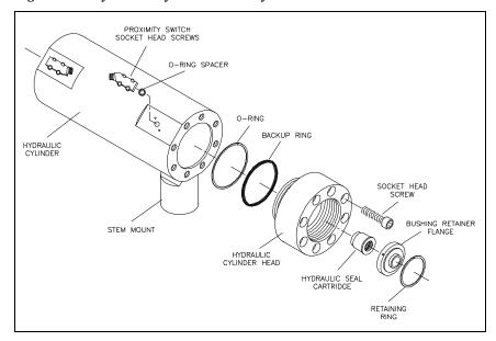
Figure 9-6: Hydraulic Piston
