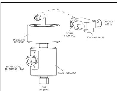
Figure 9-24: 3-Port High Pressure Dump Valve
