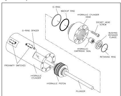
Figure 9-20: Hydraulic Piston Removal
