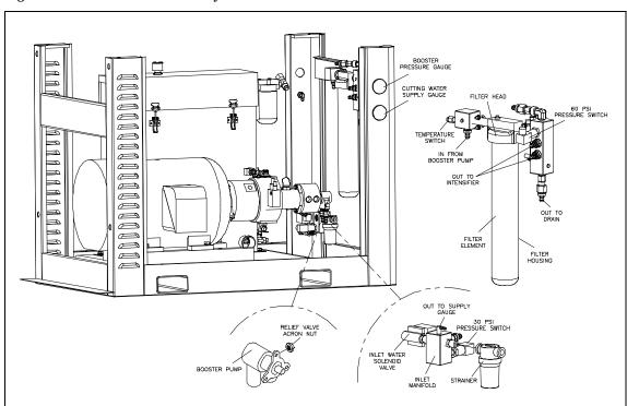
Cutting water enters through the normally closed, inlet water solenoid valve. When the control power is turned on, the solenoid valve opens and allows water to flow through the valve. The inlet water is monitored by a 30 psi pressure switch mounted on the inlet manifold. If the pressure drops below 30 psi (2 bar) the switch activates an automatic shutdown circuit in the PLC and the machine will not start.
