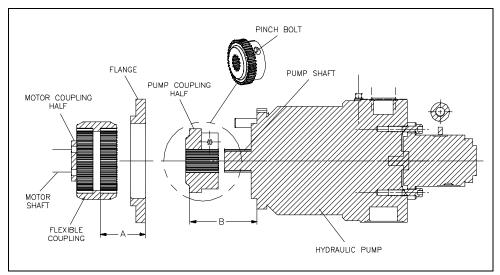
From dimension A, subtract 5/16 inch for 30, 50 and 60 horsepower motors, and 1/4 inch for 75 and 100 horsepower motors.
