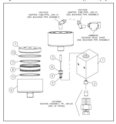
Figure 12-5: Pneumatic Valve/Actuator Assembly, Normally Open
