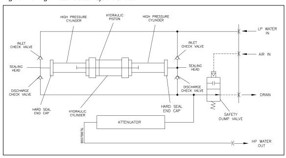
Figure 9-1: High Pressure Water System Circuit
