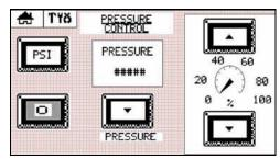
8. Check the motor rotation. Press the START button on the Run Screen and observe the pressure gauge on the hydraulic manifold. If the motor rotation is correct, pressure will begin to build in just a few seconds. If the rotation is not correct, the gauge will not move.
