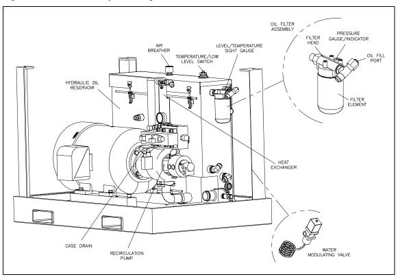
Figure 6-2: Recirculation System Components (Oil-to-Water)
