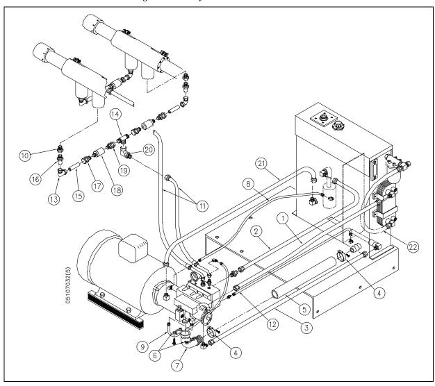
Figure 12-12: Hydraulic Hose Connections
