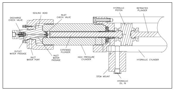
Low pressure water is routed through the inlet water ports to the inlet passages in the sealing heads. When the plunger retracts, the inlet check valve opens to allow water to fill the high pressure cylinder. When the plunger extends to create high pressure water, the inlet valve closes to seal the inlet passage and the discharge check valve opens to allow the high pressure water to exit the cylinder. As the plunger retracts, the discharge check valve closes.
