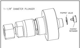
The inlet check valves should be serviced on a regular, preventive maintenance schedule. Service is recommended every 1,000 hours for units with 7/8" diameter plungers and every 1,500 hours for units with 1-1/8" diameter plungers. The hard seal end cap must be removed to service the inlet check valve. Follow the procedure, Hard Seal End Cap Removal. When the end cap has been removed, proceed with Step 1 below.
