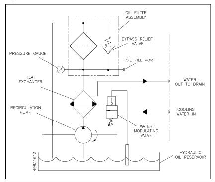
Figure 6-1: Oil Recirculation Circuit
