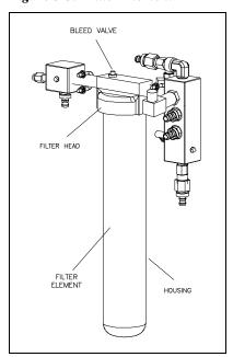
Figure 5-3: Filter Element
