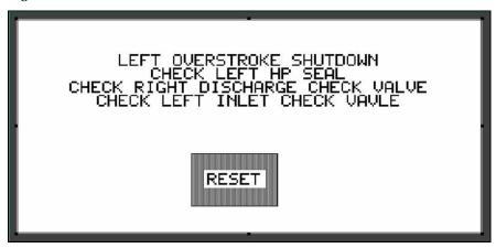
Pressing the RESET button will clear the alarm banner, but it will not clear the fault. The banner will continue to display until the fault is corrected. Shutdowns will appear on the Alarm History Screen. Alarm banner shutdowns are listed in Table 4-4.
