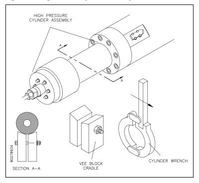
Figure 9-8: High Pressure Cylinder Assembly Removal and Installation
