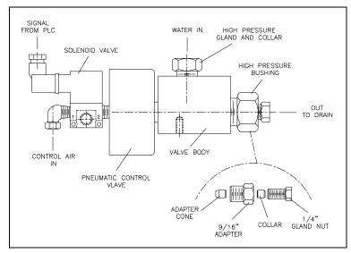
Figure 9-28: 2-Port High Pressure Dump Valve
