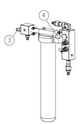
A temperature switch monitors the temperature of the cutting water from the booster pump. If the temperature exceeds 128° F (53° C), the switch activates an automatic shutdown circuit in the PLC. The temperature switch prevents booster pump overheating due to lack of water, long deadhead conditions or a blocked orifice.
