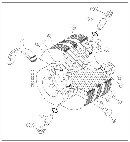
Figure 12-6: Hydraulic Piston Assembly
