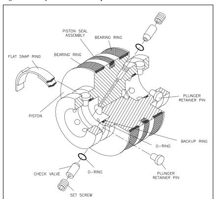
Figure 9-19: Hydraulic Piston Components
