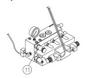
Optional proportional pressure control allows the operator to select or vary the hydraulic operating pressure from the control panel or from a remote console. An electronically controlled hydraulic cartridge valve, mounted on the hydraulic manifold, receives a signal from the PLC and automatically
