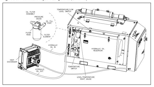
Figure 6-3: Recirculation System Components (Oil-to-Air)
