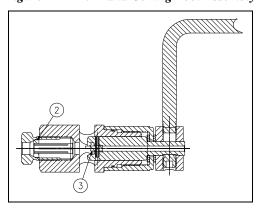
Figure 12-21B: Power Coning Tool Assembly
