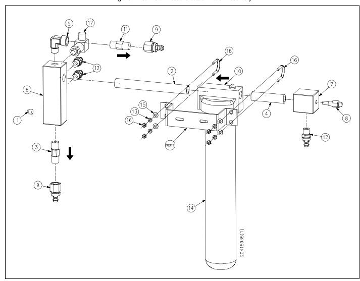
Figure 12-8: Low Pressure Water Filter Assembly
