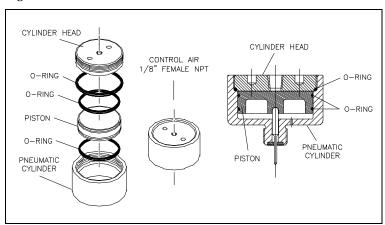
1. Unscrew and remove the cylinder head using a strap wrench and a pin spanner. Remove the piston from the cylinder.
