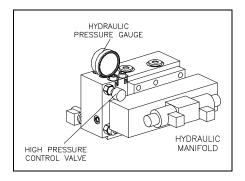
If the machine is equipped with proportional pressure control, the high pressure adjustment is made from the Pressure Control Screen on the control panel. Refer to Section 4, Operation, for additional information.
