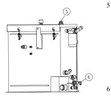
The temperature/low level switch monitors the oil temperature and level in the reservoir. Although the float switch and the temperature switch are combined in a single unit, the two switches function independently.
